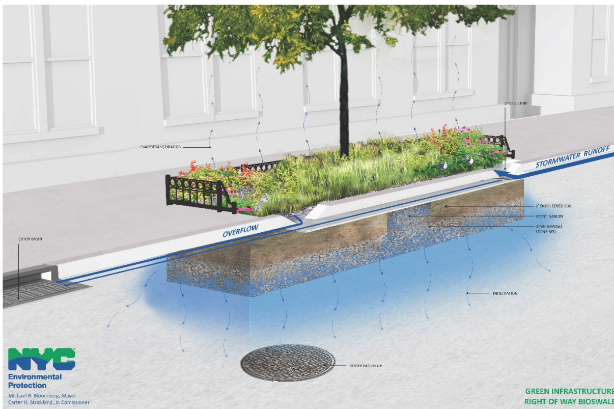
Figure 1-1. Standard Right-of-Way Green Infrastructure
