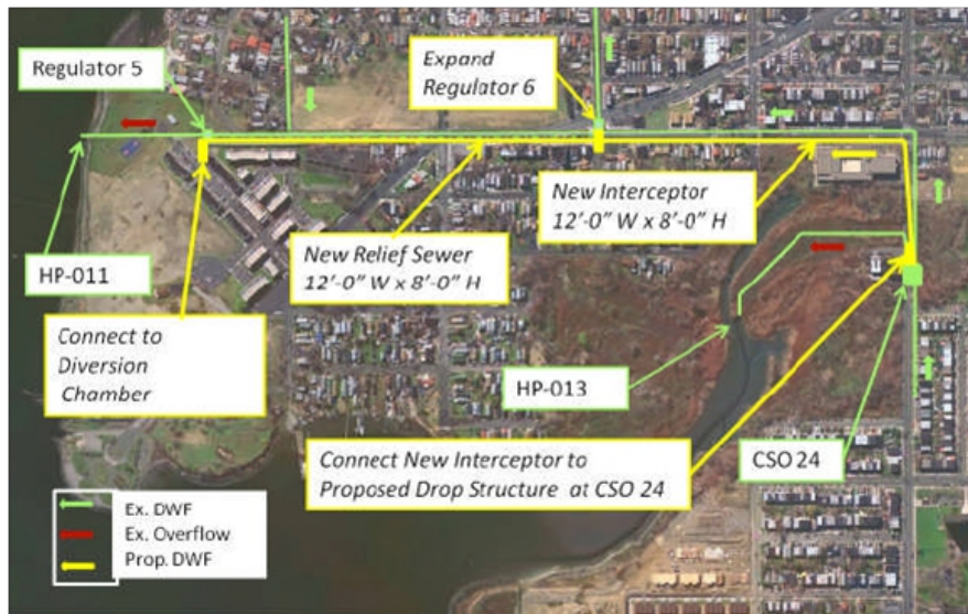
Concept 3. Parallel Relief Sewer
