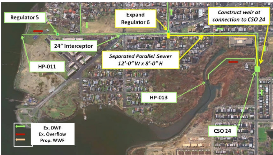
Concept 2. Wet Weather Parallel Sewer
