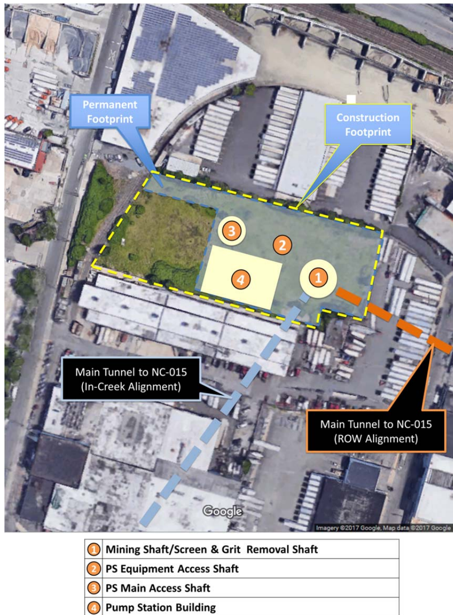
Figure 8-18. Conceptual Layout of Mining Shaft/TDPS at DEP Owned Parcel – Shorter Tunnel
