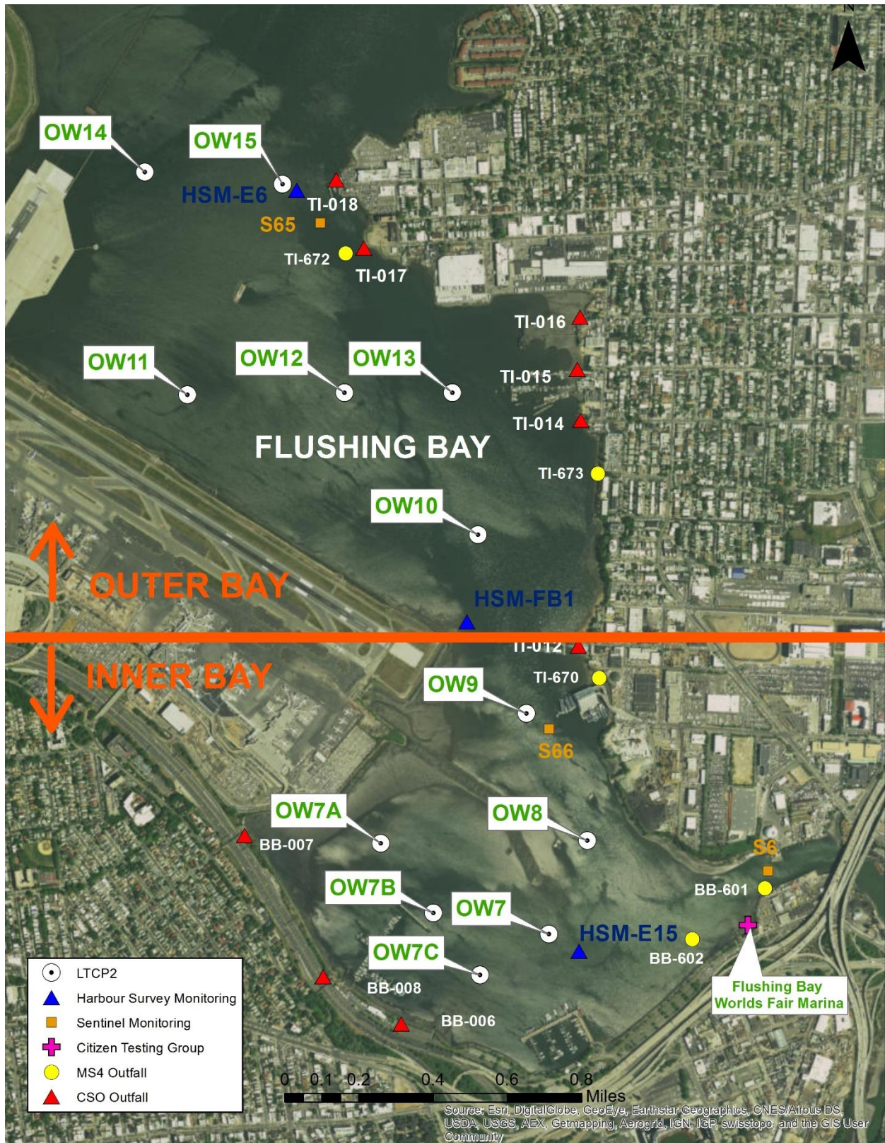
Figure 6-2. LTCP2 Water Quality Monitoring Stations in Flushing Bay
