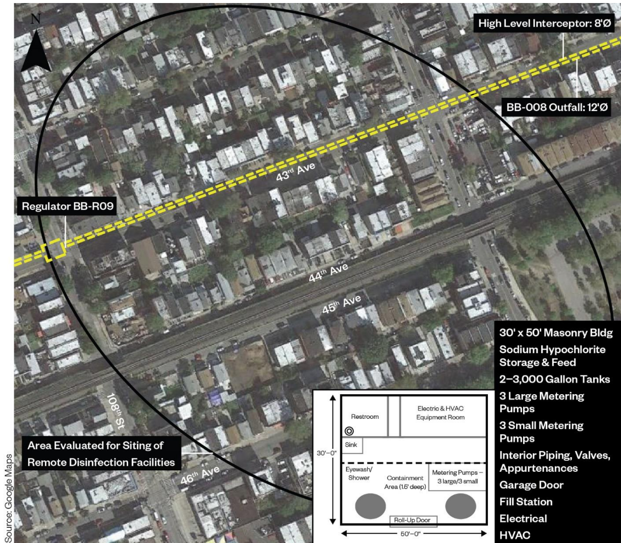
Figure 8-14. Alternative 9-1 – Remote Disinfection Facility for Outfall BB-008
