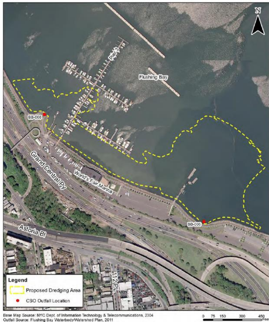
Figure 4-3. Dredging Location in Flushing Bay
