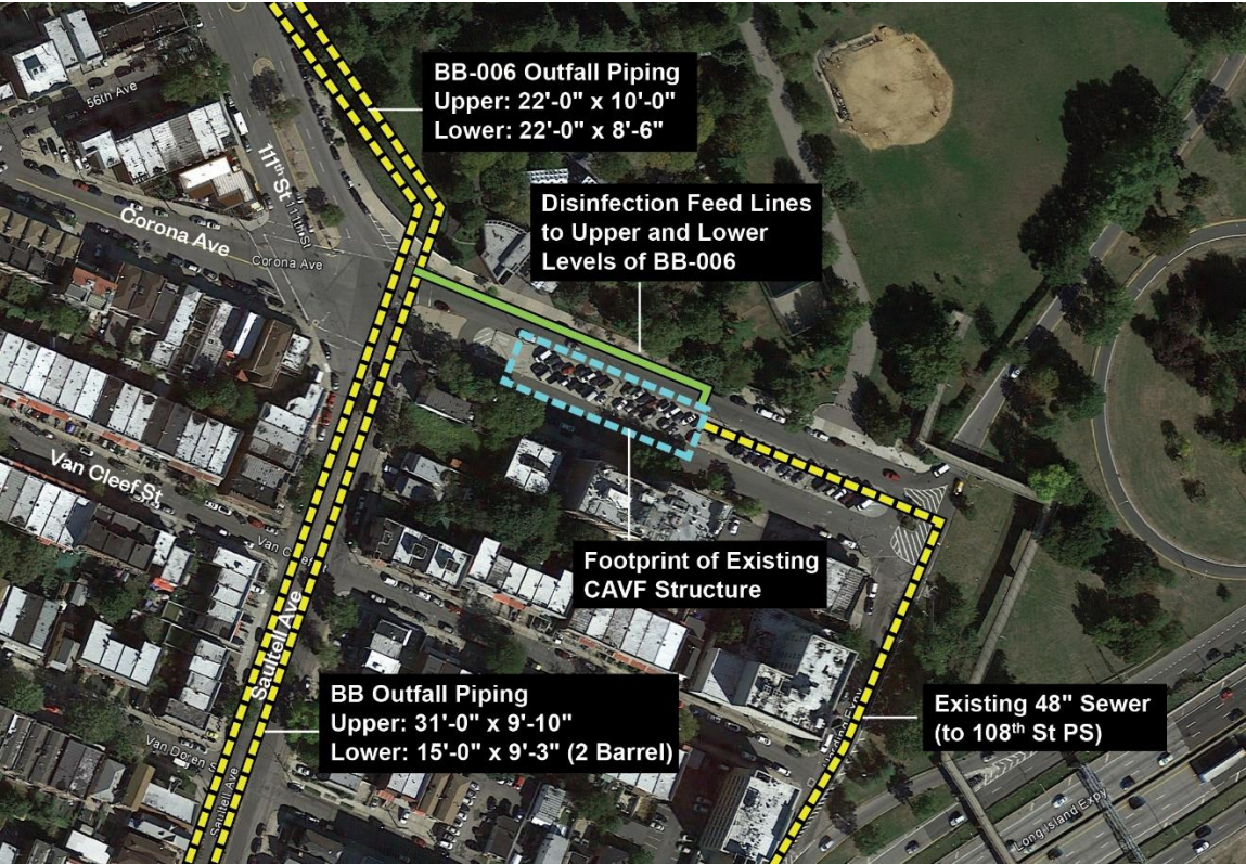
Figure 8-13. Alternative 9-1 – Retrofit of CAVF for Disinfection of Outfall BB-006
