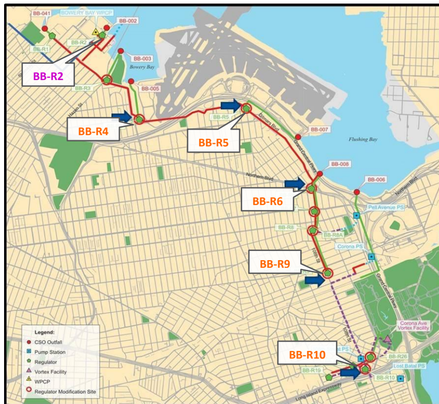
Figure 4-2. Flushing Bay High Level Interceptor Regulator Improvements
