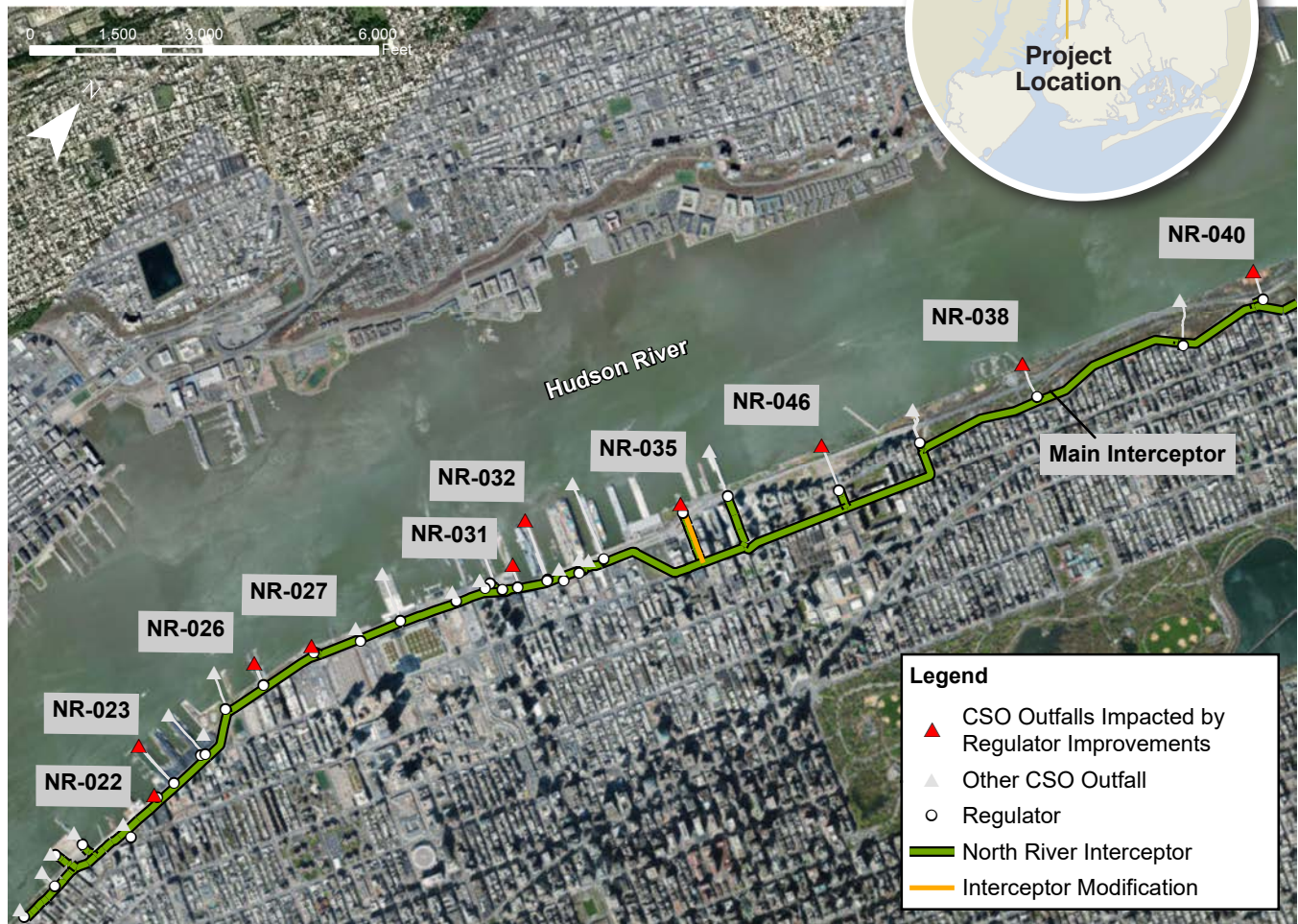
Location of the regulators to be modified under HUD-1 and HUD-2
