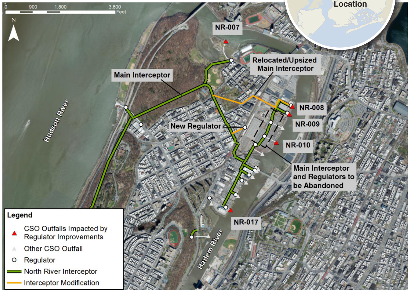
Location of the regulators to be modified under HAR-1 and HAR-2
