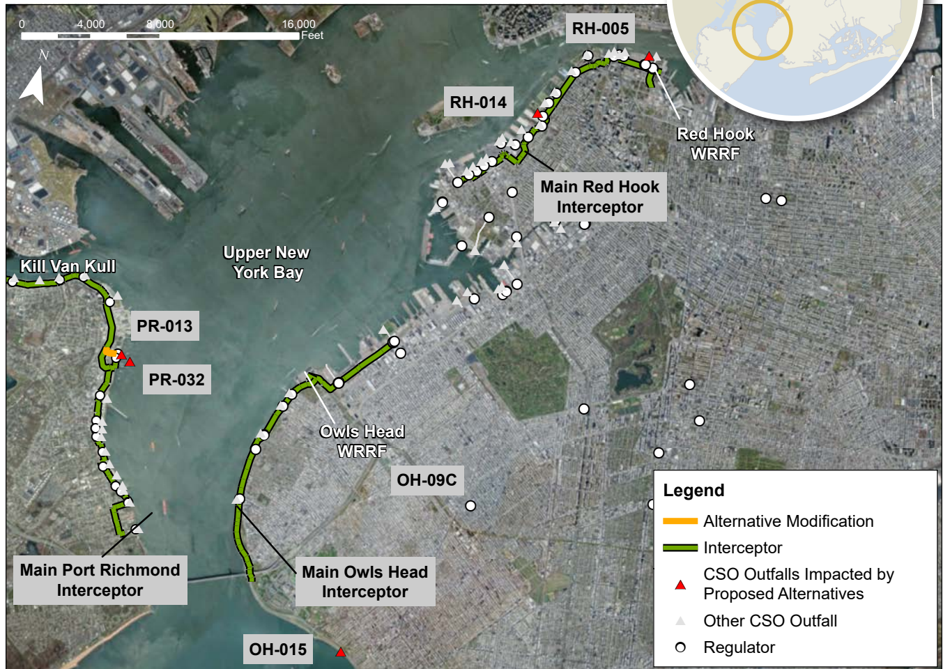
Location of the regulators to be modified under NYB-1 and NYB-3, and location of bypass pipe for NYB-2
