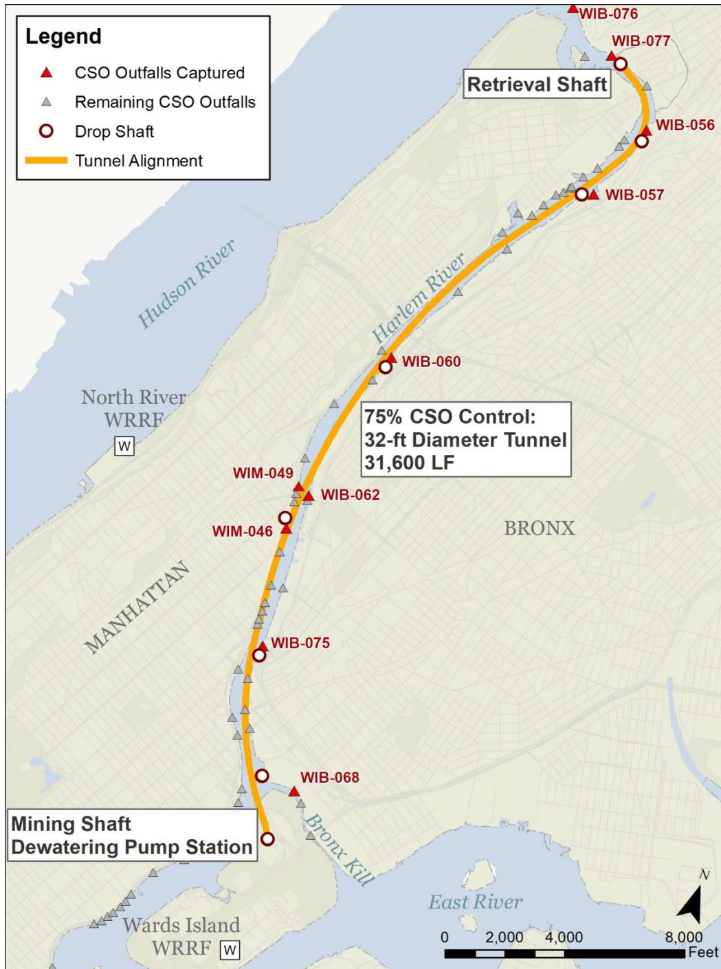
Figure 8.3-7. Conceptual Layout for 75% Control Storage Tunnel for Harlem River
