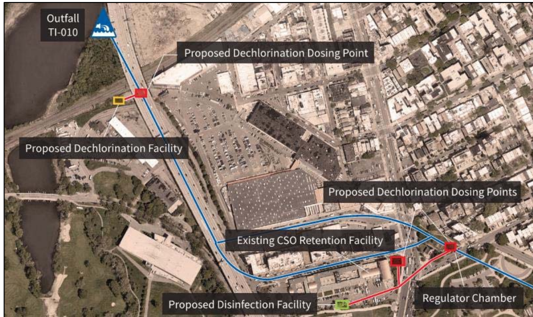
Figure 4-12. Seasonal Disinfection at Flushing Bay CSO Retention Facility and Diversion Chamber 5
