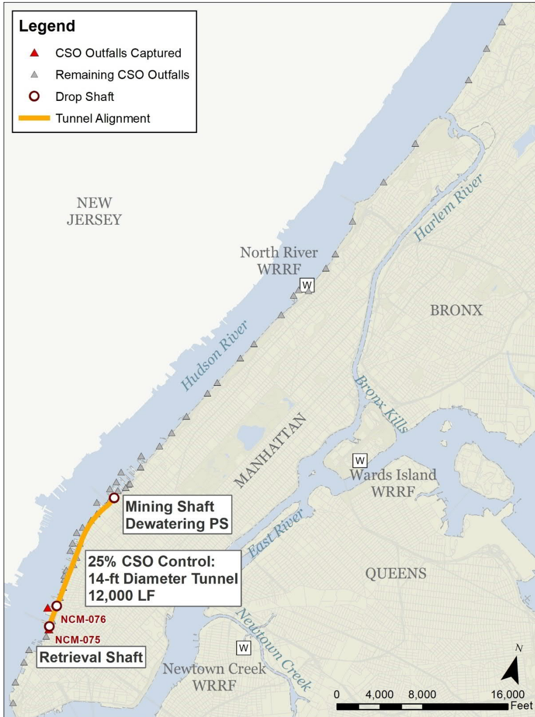
Figure 8.4-6. 25 Percent CSO Control Tunnel for Hudson River
