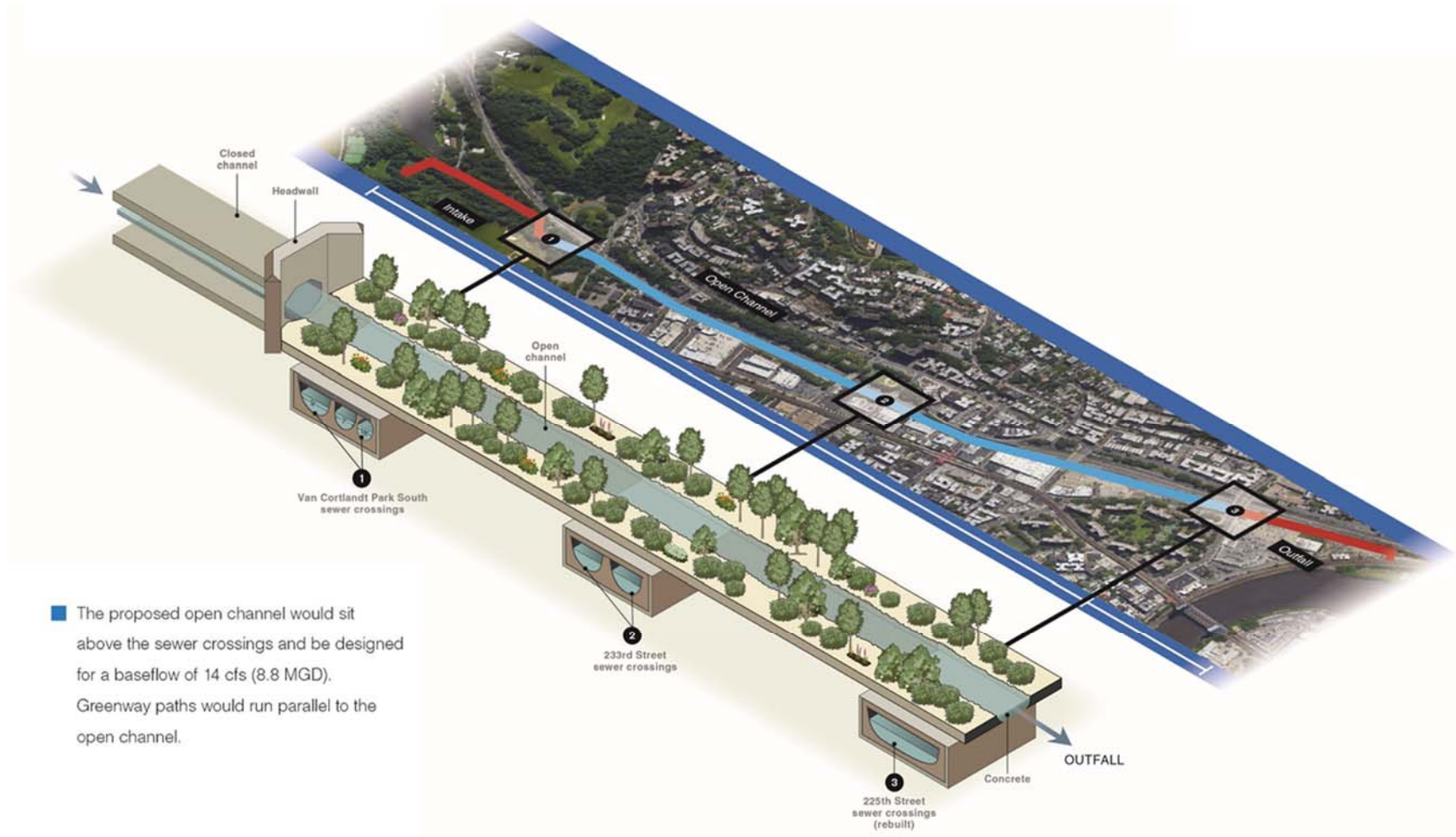
Figure 5-4. Location of Sewer Crossings along the Proposed Route of Tibbetts Brook Daylighting
