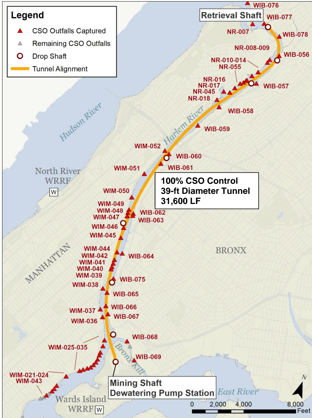
Figure 8.3-8. Conceptual Layout for 100% Control Storage Tunnel for Harlem River
