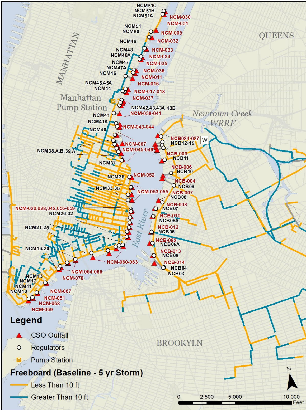
Figure 8.5-14. Hydraulic Grade Line Impacts of Newtown Creek Collection System Under Baseline Conditions (5-Year Storm)
