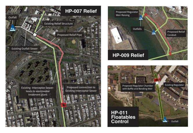
Figure 4-16. Hydraulic Relief at CSO Outfalls HP-007 and HP-009 and Floatables Control at CSO Outfall HP-011
