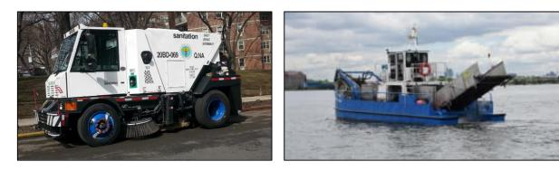
Figure 8.2-1. Examples of Mechanical Broom Truck and Skimmer Vessel
