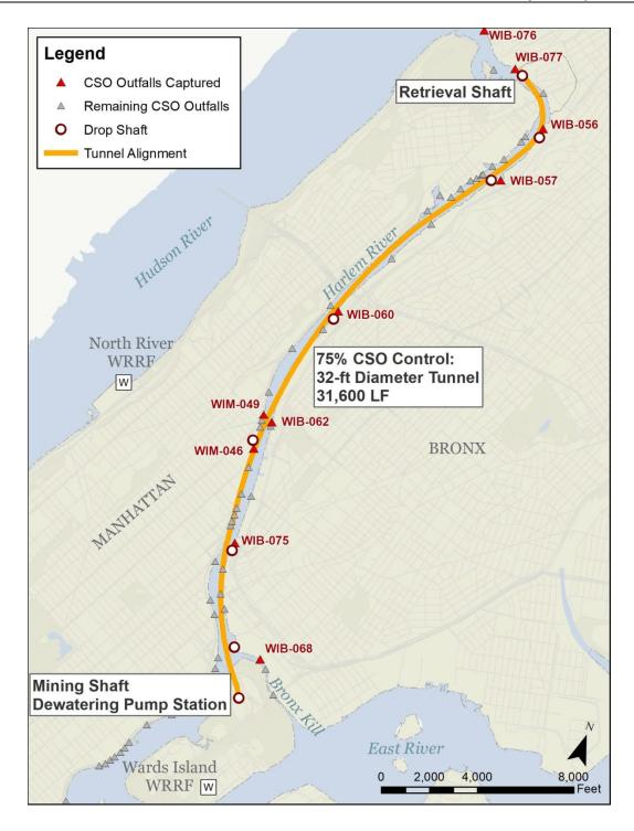
Figure 8.3-7. Conceptual Layout for 75% Control Storage Tunnel for Harlem River
