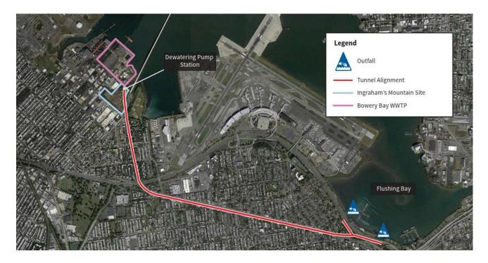
Figure 4-24. 25 MG CSO Storage Tunnel (Outfalls: BB-006 and BB-008)
