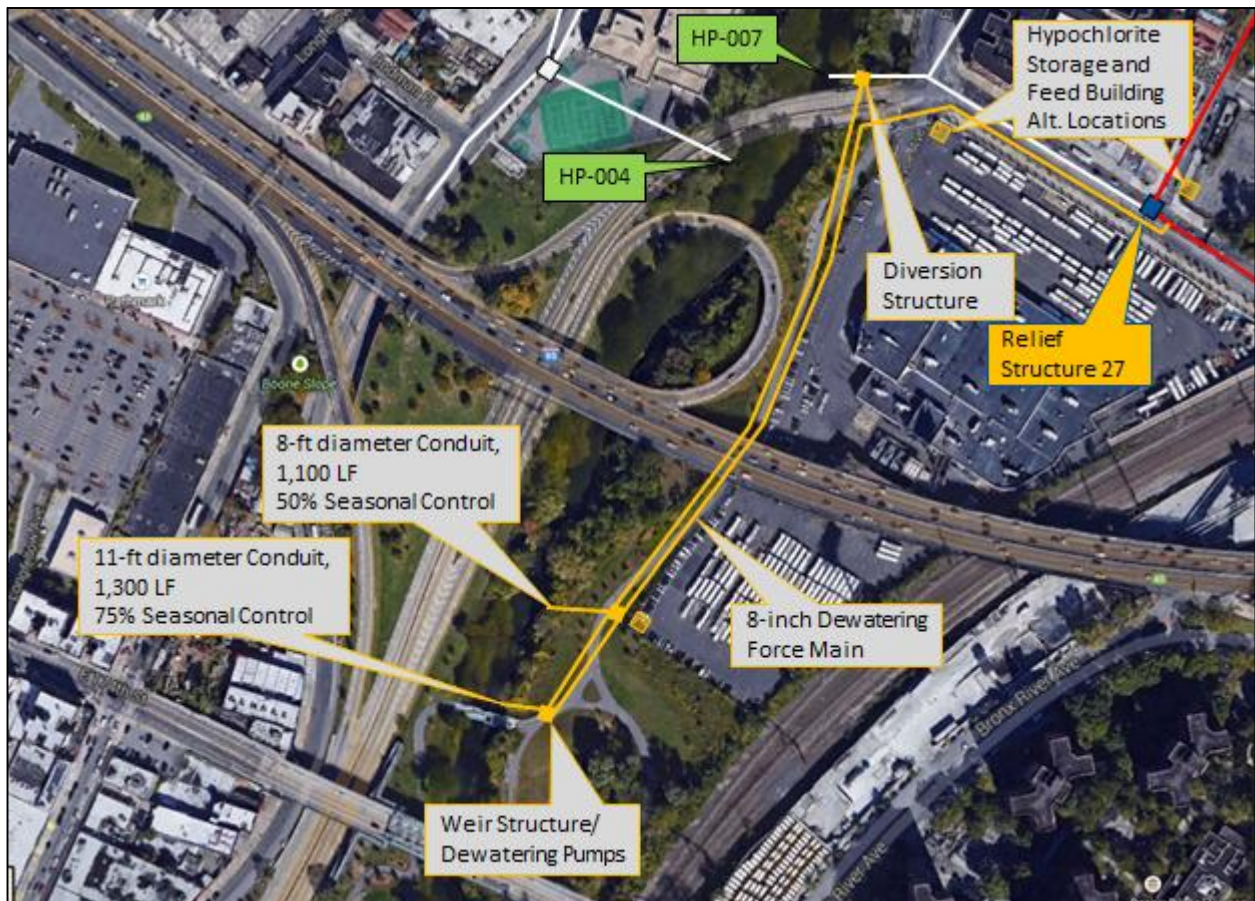
Figure 8-12. Layout of Alternative 7-2 – HP-007 Outfall Conduit Disinfection
