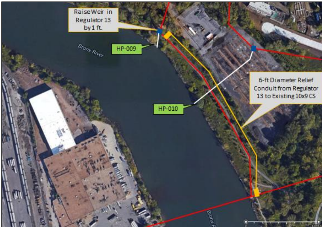
Figure 8-30. Layout of Alternative 9-1 – Hydraulic Relief of Regulator 13
