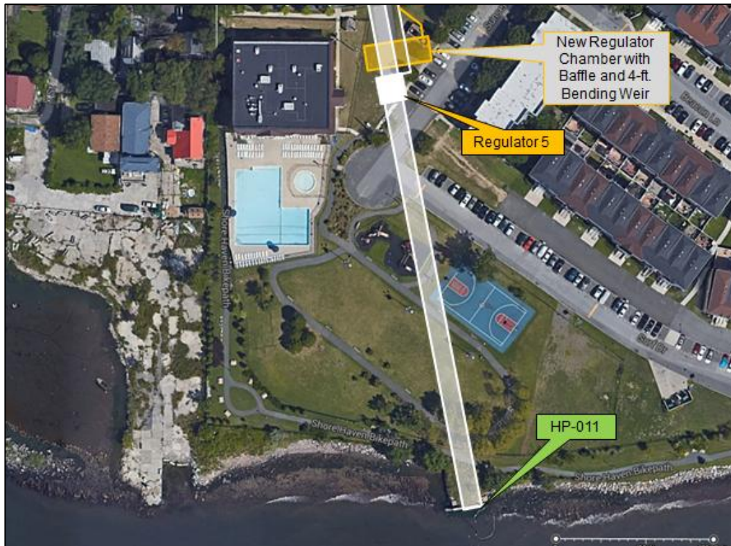
Figure 8-31. Layout of Alternative 11-1 – Regulator 5 Modification
