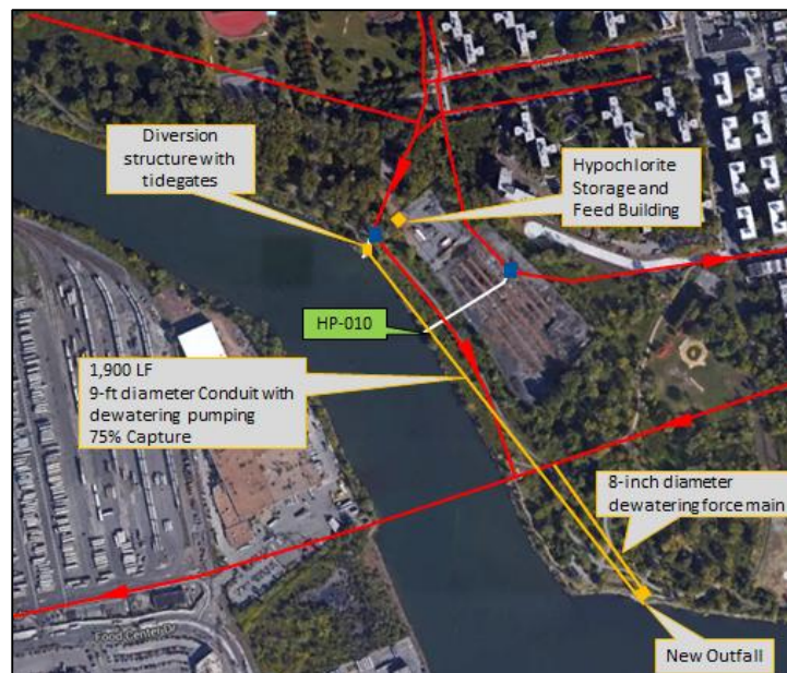
Figure 8-18. Alternative 9-3 – HP-009 Outfall Conduit Disinfection
