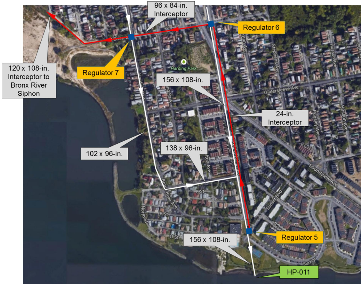
Figure 8-2. System Configuration Upstream of Outfall HP-011
