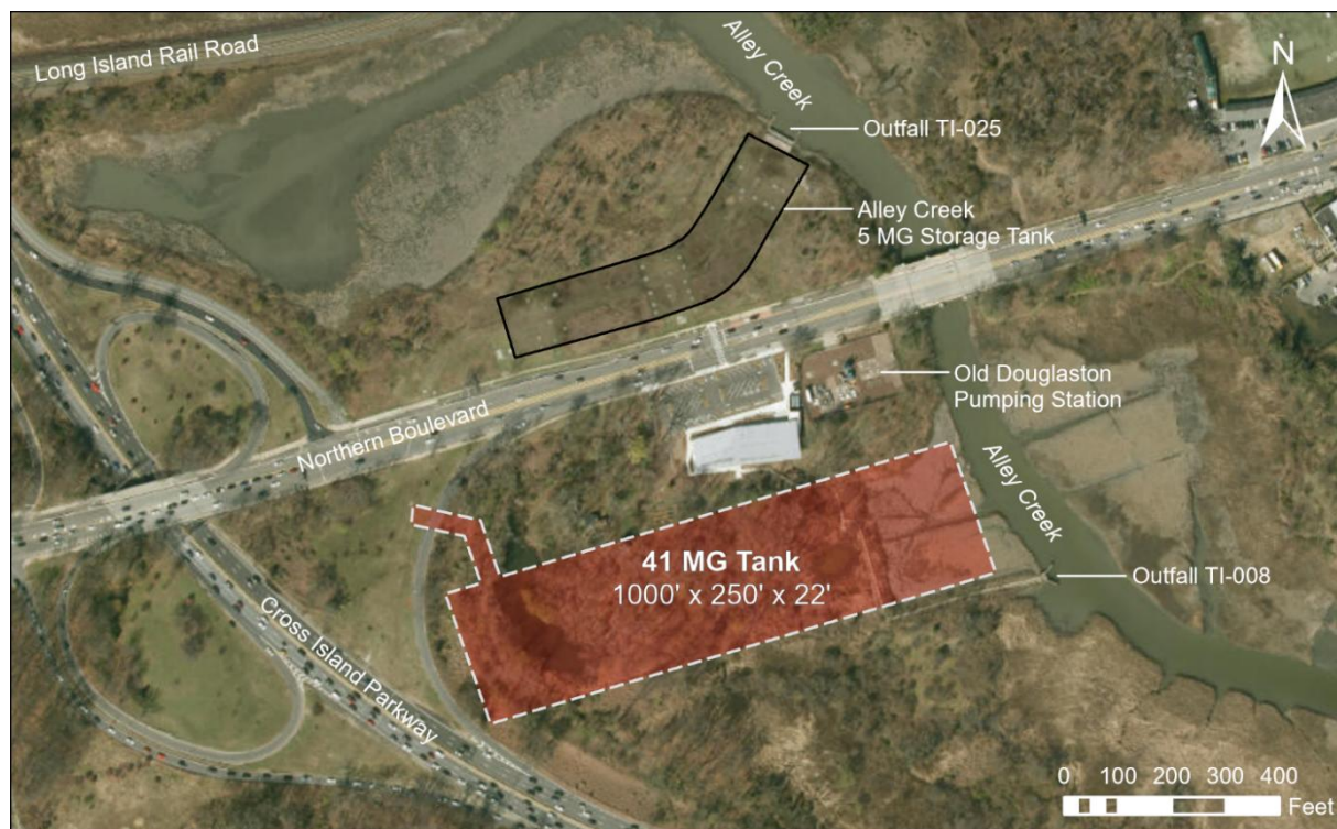
Figure 8-5. Alternative 2D – 41 MG Downstream Tank Dewatering Considerations
