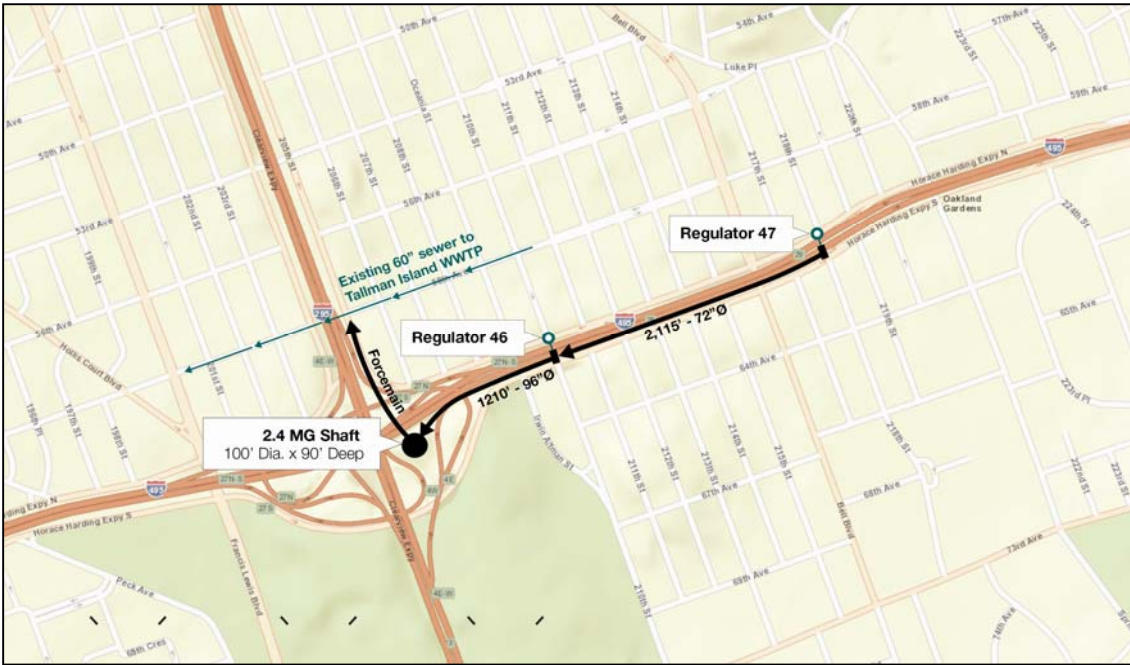
Figure 8-9. Alternative 3A – 2.4 MG Upstream Tank
