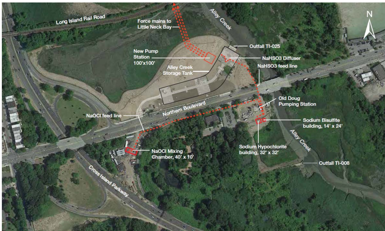
Figure 8-18. Alley Creek Tank Overflow Effluent Pump Station for Alternative 4
