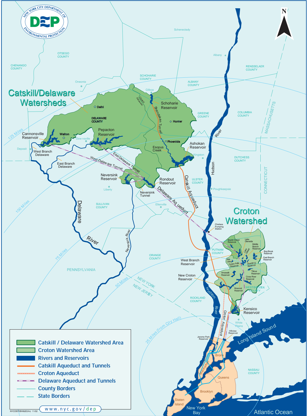
Figure ES-1 New York City Water Supply System
