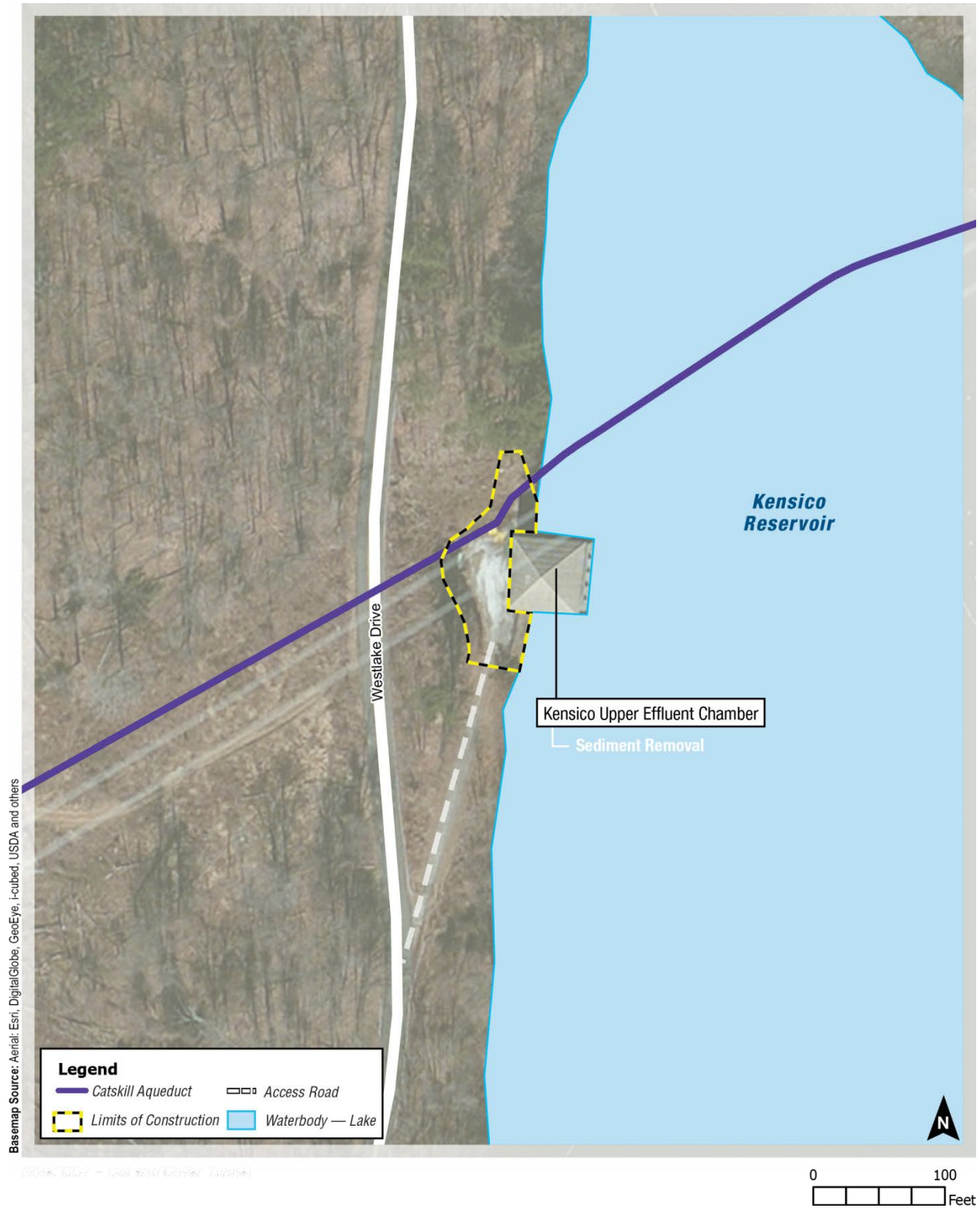
Figure 9.16-31: Site Plan for Kensico Upper Effluent Chamber – Westlake Drive Study Area
