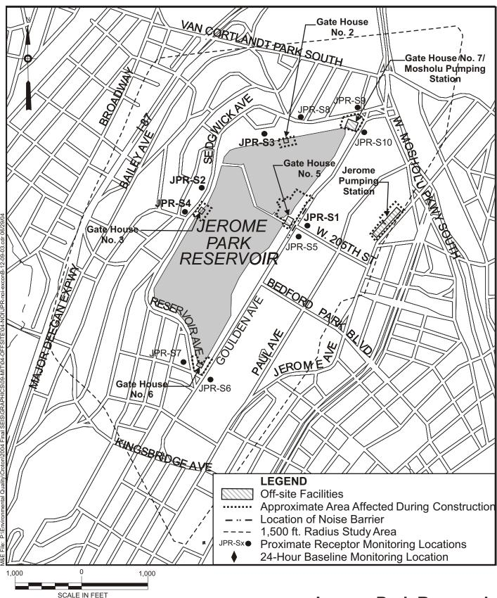
Jerome Park Reservoir Stationary Noise Source Potential Noise Barrier Configuration The equipment usage and the number of personnel working at the Shaft Site would not fluctuate substantially over the duration of the construction schedule. As a result, noise levels at the site are not anticipated to vary and any noise-mitigation requirements would be constant for the entirety of the construction schedule.
