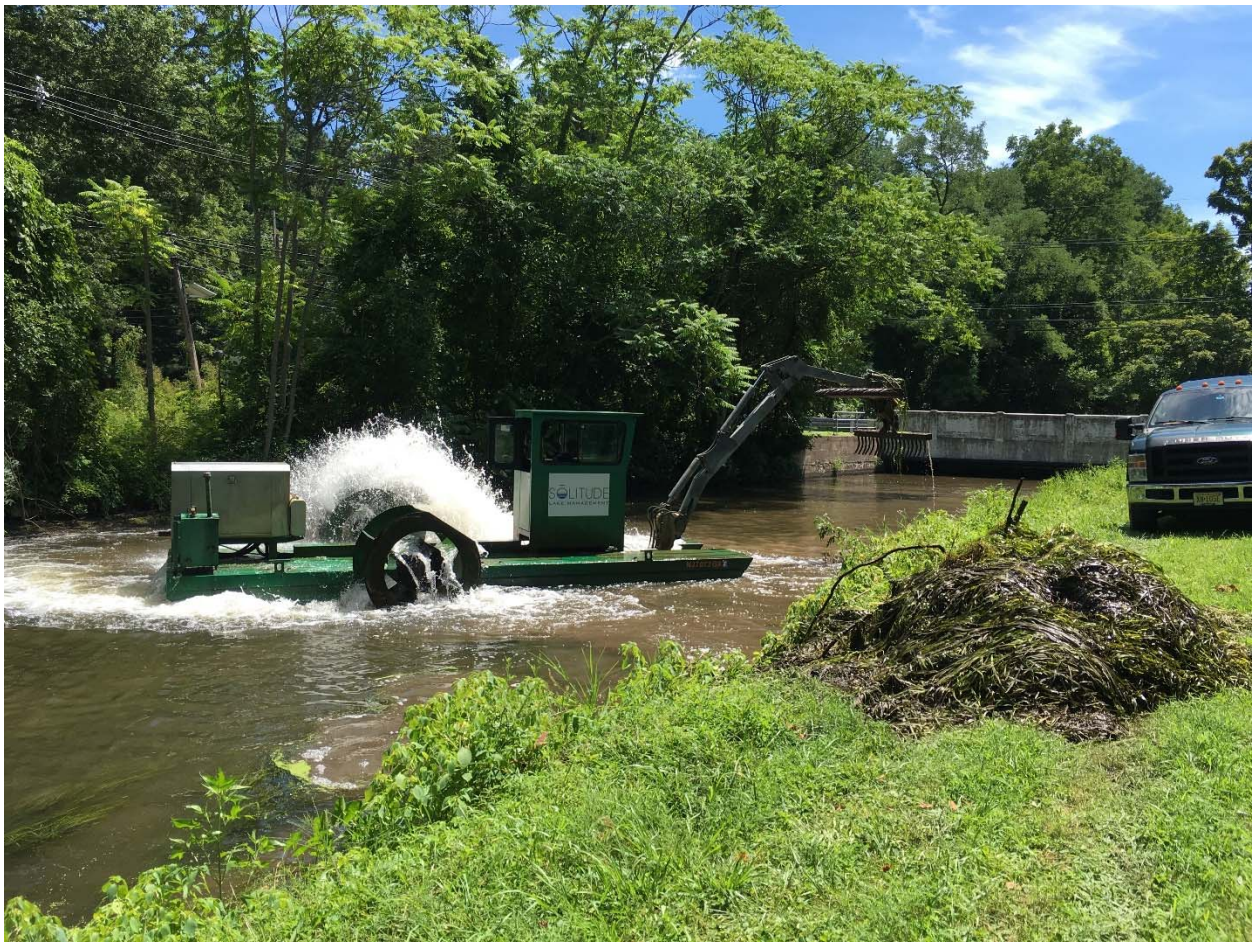
Source: Courtesy of Heather Desko/New Jersey Water Supply Authority. Figure 3 Hydroraking submersed aquatic plants in the D&R Canal
