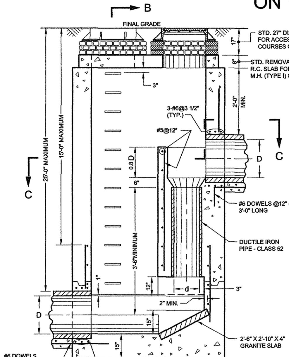
STD. 27" DIA. M.H. FRAMES AND COVERS FOR ACCESS AND CLEANOUT ON THREE COURSES OF BRICK LAID RADIALLY
