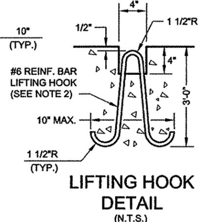
LIFTING HOOK DETAIL (N.T.S.)
