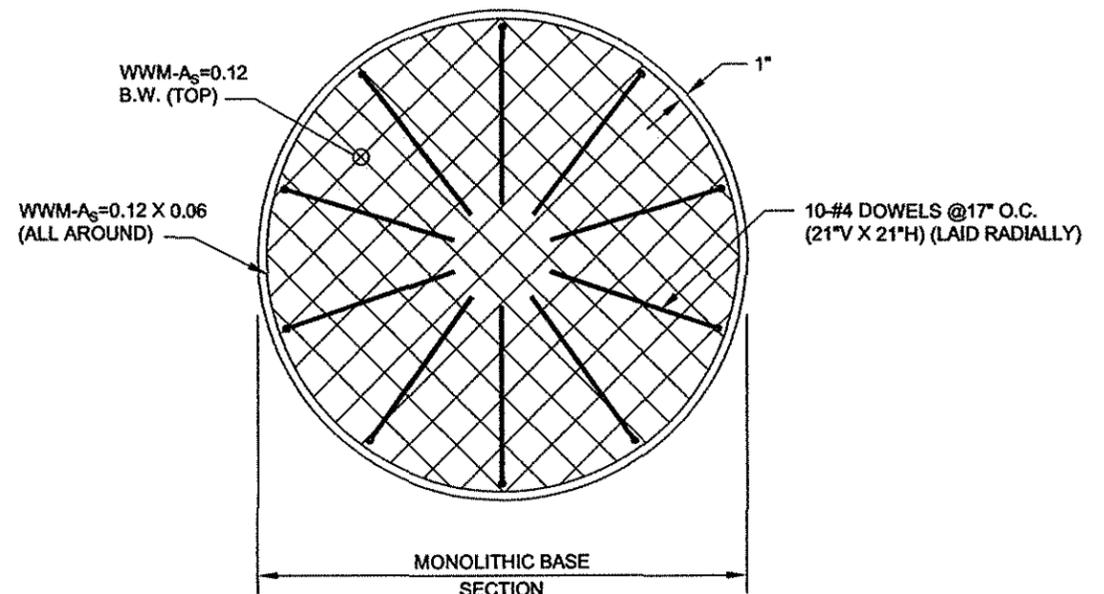
PLAN OF BOTTOM REINFORCING SECTION
