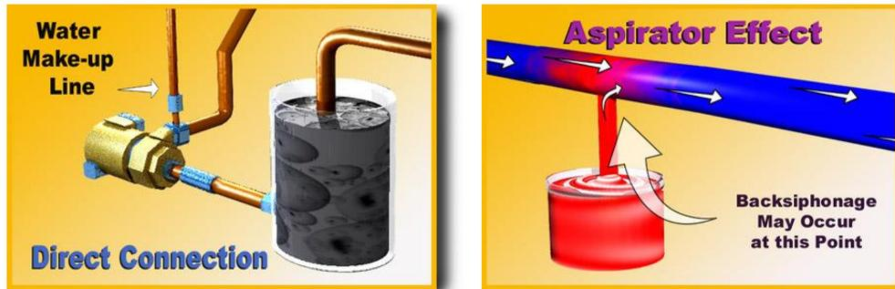
A cross-connection is any actual or potential physical connection between a potable water line and any pipe, vessel, or machine containing a non-potable fluid, or has the possibility of containing a non-potable fluid, solid or gas, such that it is possible for the non-potable fluid, solid or gas to enter the potable water system by backflow.
