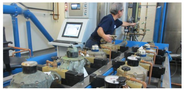
At our Meter Test Facility, DEP employees carry out critical testing and upkeep to monitor the accuracy and coordinate necessary repairs of our water meters.
