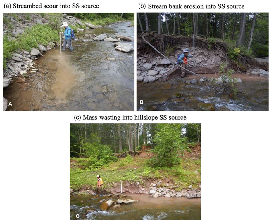
FIGURE 3 Examples of the types of erosion in the Stony Clove sub-basin (NYC DEP, 2019a)
