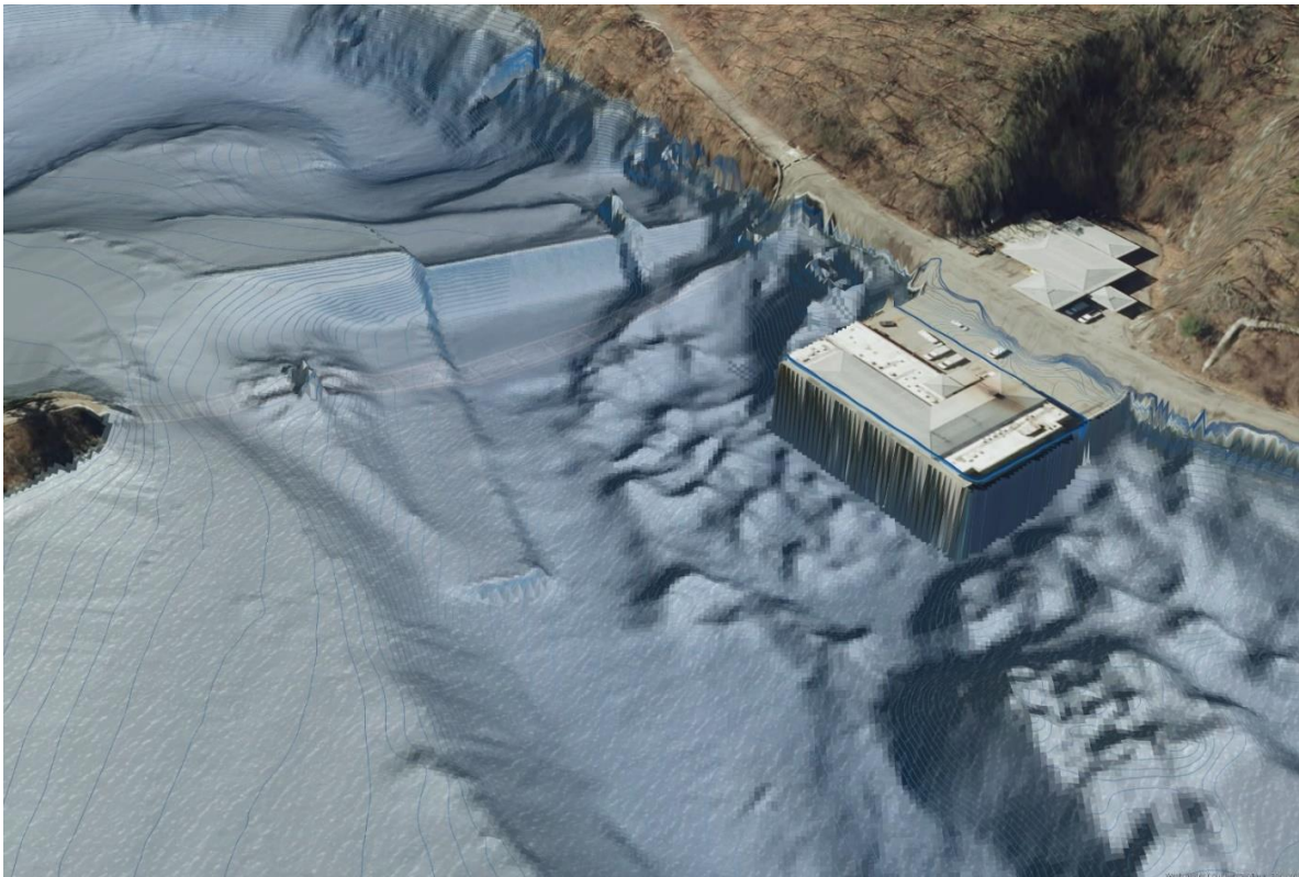
Figure 5.3 Topographic surfaces derived from sonar-generated bathymetry are used to render a 3-dimensional view of the submerged Old Croton Dam near the Croton Lake Gatehouse. USGS developed these high-resolution bathymetry data for each EOH reservoir.
