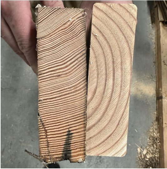
Figure 5. Old-growth Wood (left) and Modern Wood (right)
