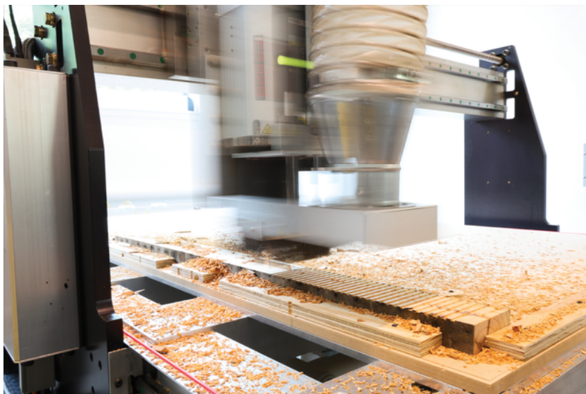
Figure 31. CNC - GrooveLam (Cornell Circular Construction Lab, 2022)
