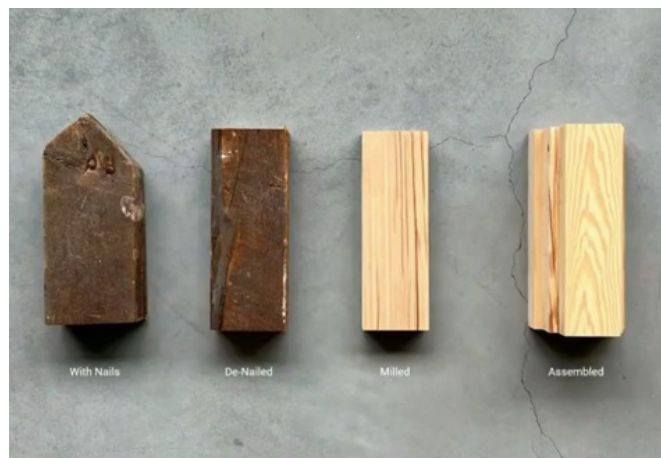
Figure 4. Life Cycle of Reclaimed Wood (CO Adaptive, 2026)
