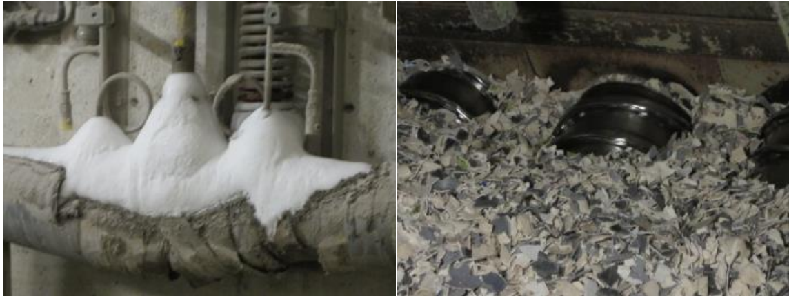
Figure 3: PVC Chip (30mm) and Finely-Ground Particle (<0.4mm) Processing (Goedecke, 2016)
