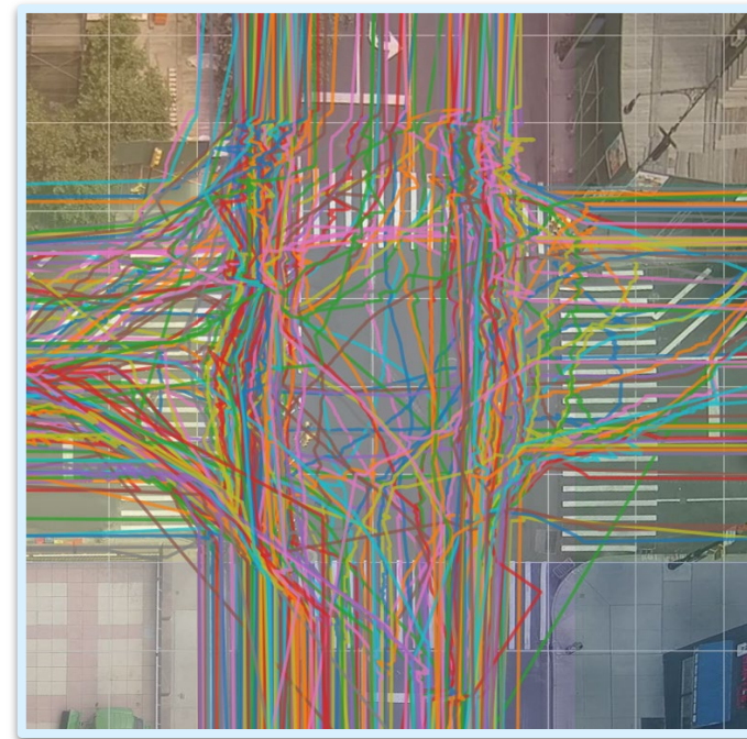
Figure: Sample plot of collected e-bike tracks in bird's-eye view.
