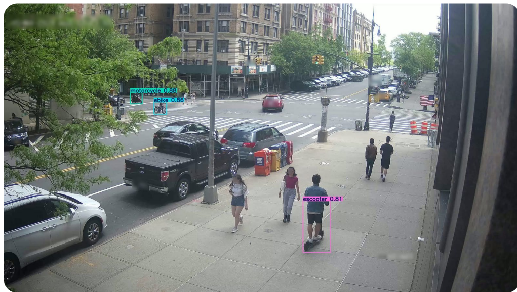
Figure: Real-time object detection and tracking for micromobility classes.
