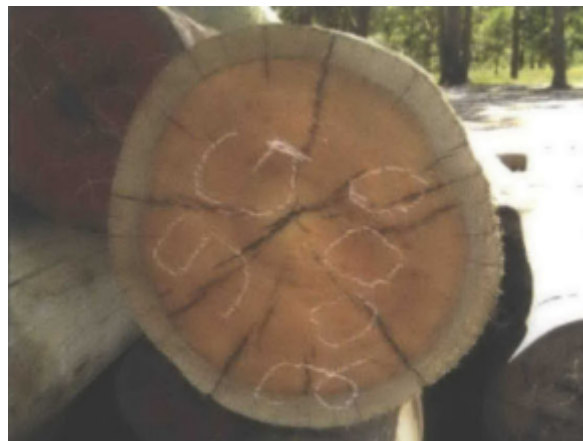
Figure 8. Cross-section of a chromated copper arsenate (CCA)-treated utility pole, illustrating preservative penetration patterns within treated wood. This figure highlights the health and regulatory concerns associated with reusing chemically treated lumber, which restrict its application primarily to non-residential or exterior uses.
