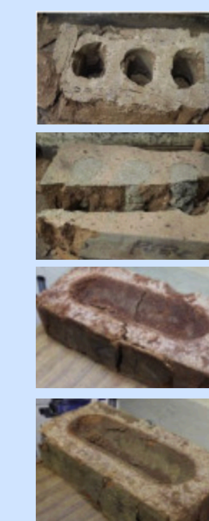
Figure 3. from top to bottom: reclaimed perforated (no infill), with infill, new frogged, reclaimed frogged
