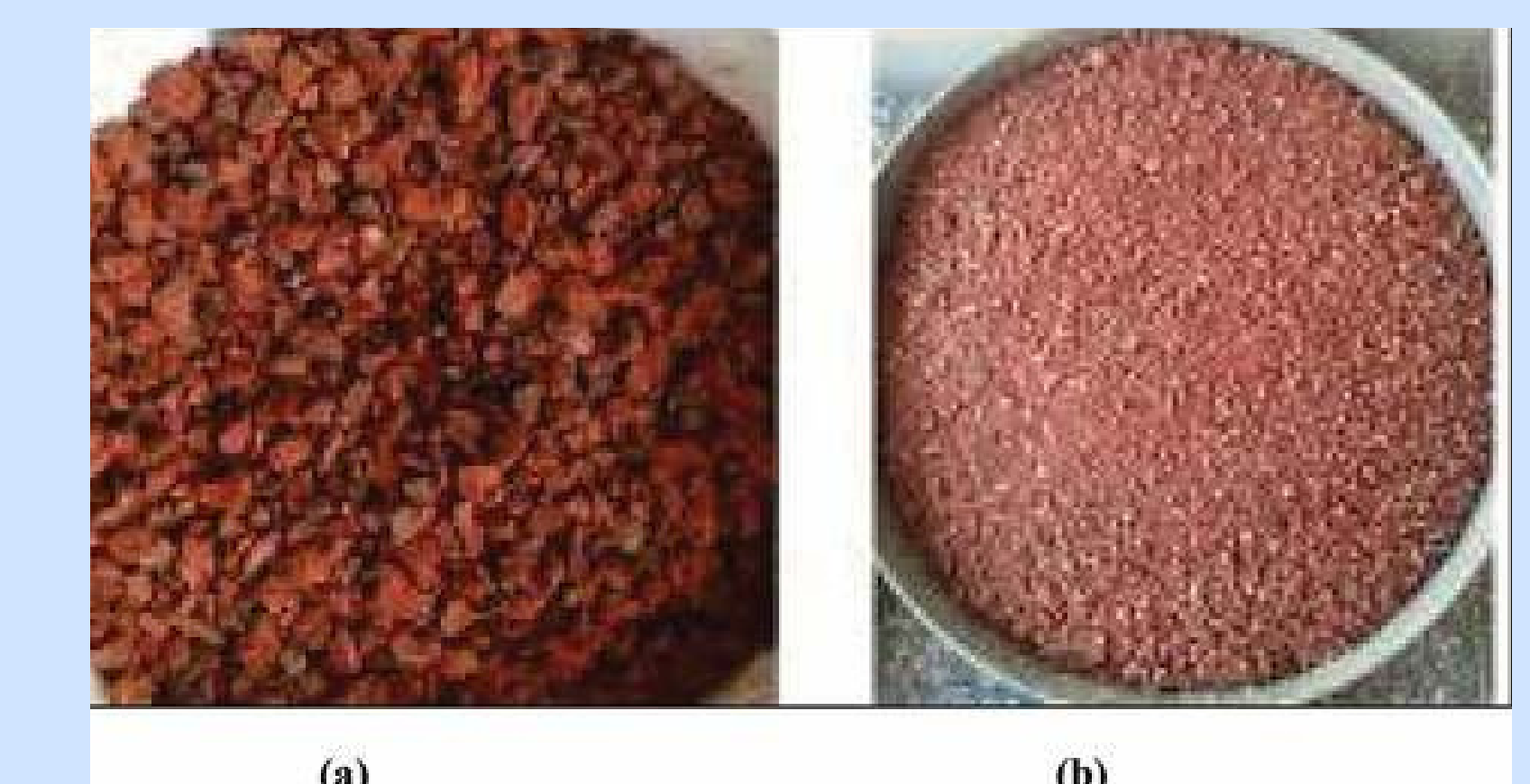
Figure 8. Crushed clay bricks as fine aggregate for a) concrete and b) cement mortar
