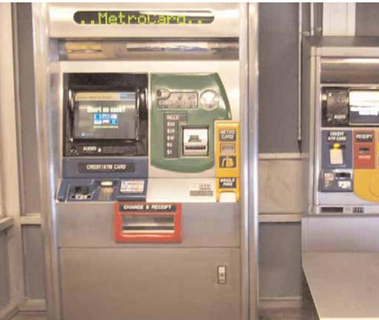
Information Transaction Machines (ITMs) include any **interactive terminal in which the primary purpose is to accept input from a user, display information, and/or dispense media.** Such machines include automatic teller machines or cash machines, postage stamp dispensers, fare machines, automated airport check-in machines, and information kiosks.
