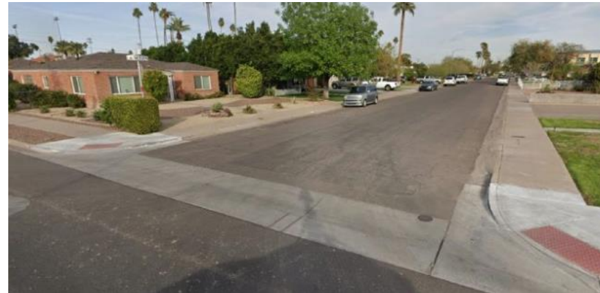
Depressed Gutter Gutter across intersections
