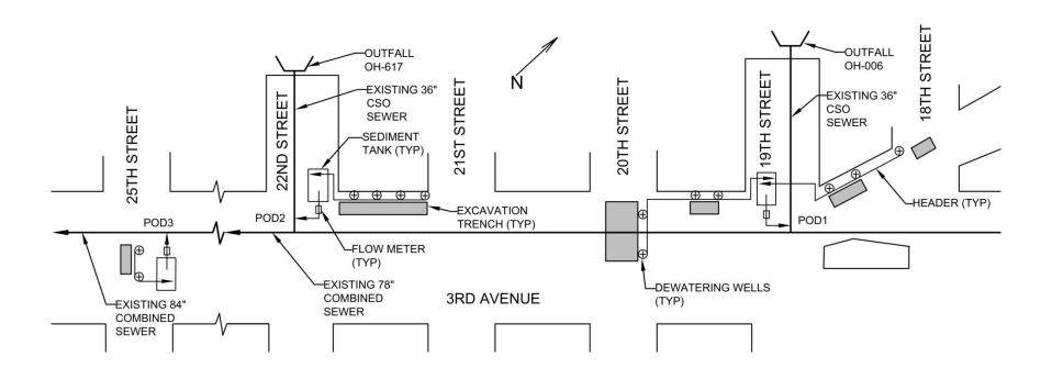
Figure 2: Groundwater Discharge Locations and Flow Diagram
