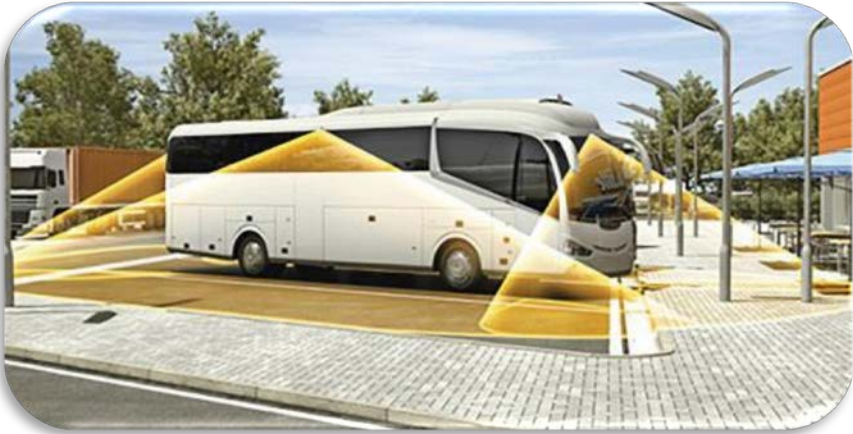
External Camera Placement
