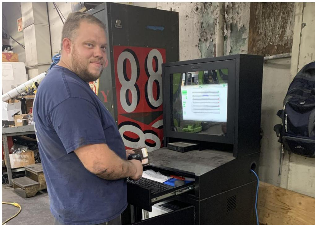
The new system employs wireless technology, updated analyzers, on-board diagnostics (OBD), and printers for stickers. Installation and training on these units was time-consuming for all the garages. All commercial garages in the state also were required to do this update.
