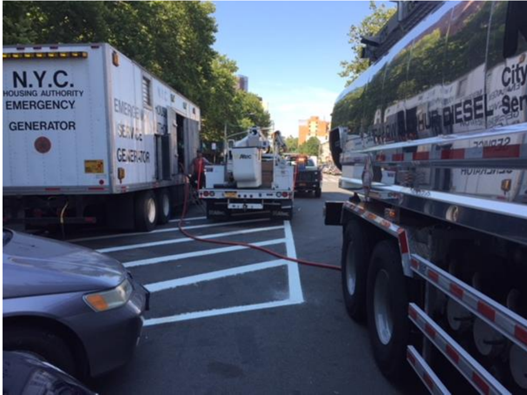
DCAS fuel truck providing emergency generator support to NYCHA.
