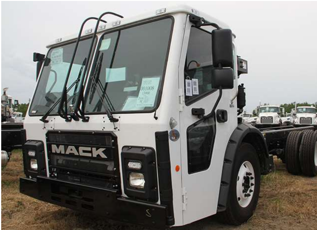
Figure 7: Example available high vision cab model: Mack LR. However, note that the A pillars and associated blind spots appear wider than the other other low-entry cabover examples.
