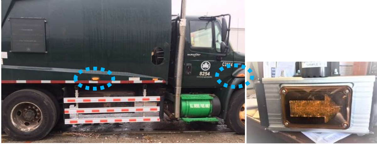
Figure 13. Side-visible turn signals on a Parks truck (left) and an audio-visual turn signal tested by NYCDOT (right).
