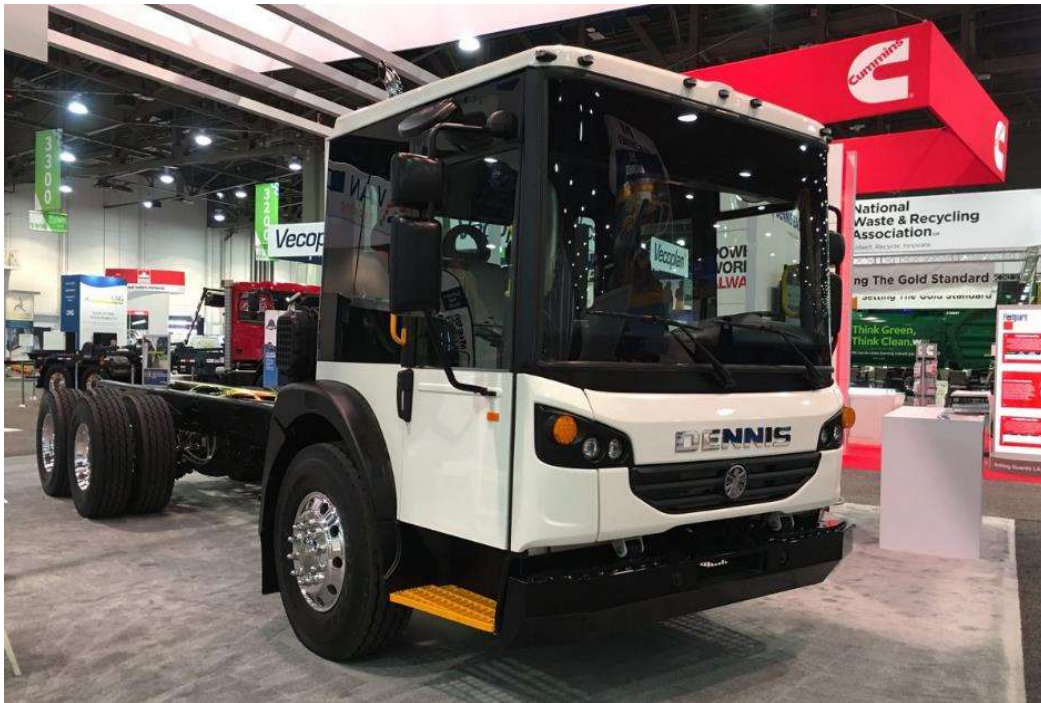
Figure 5: Example available high vision cab model: Dennis Eagle Proview
