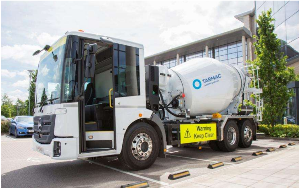
Figure 6: Example high vision cab model implemented as a mixer: Mercedes Benz Econic, equivalent to Freighliner EconicSD
