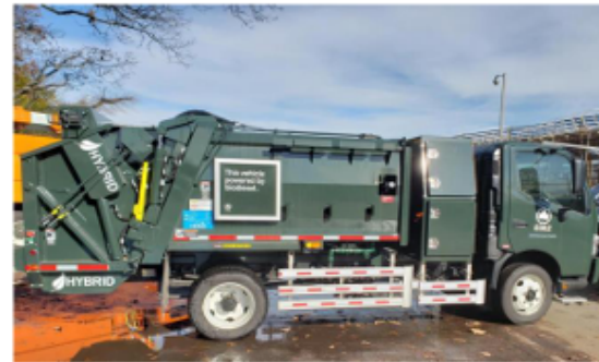
NYC Department of Parks and Recreation garbage truck powered by biodiesel and a hybrid electric drive train.
