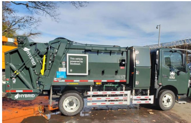
NYC Department of Parks and Recreation garbage truck powered by biodiesel and a hybrid electric drive train.
