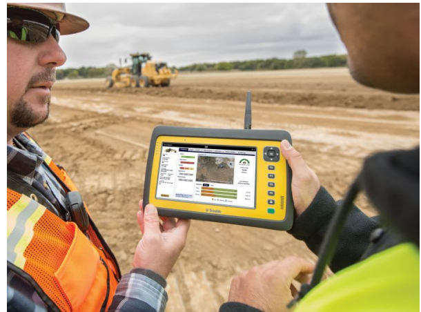
Figure 4. Caterpillar telematics system monitors real-time telematics data, including fuel levels, engine performance, and hydraulic pressure.
