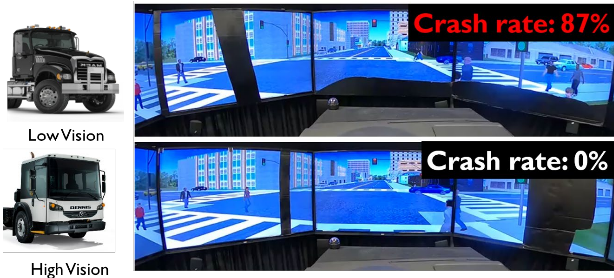
Figure 7. Vehicles simulated in Volpe research for blind zone crash outcomes with a person in the crosswalk at a signalized intersection
