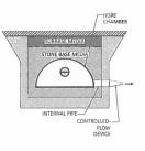
Blue roof – any rooftop that is outfit with a system that temporarily holds back water on the roof surface. Common
