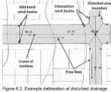
areas with separation lines for the crown of roadway and catch basins
