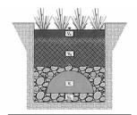
During the design process, designers should also consider any other factors which may impact the size of the overall practice or specific elements. For example, the elevation of the overflow device will govern the top of the active storage zone, which may impact the depth of drainage media that may be counted towards SMP storage volume.
