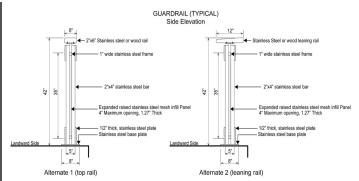
All guardrail components and hardware shall be in unpainted stainless steel and shall conform to any additional standards set forth by DPR.
