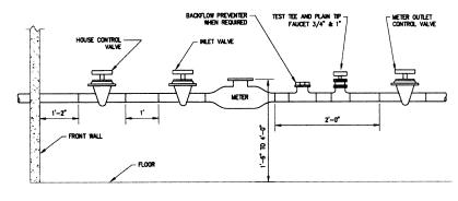
1"-2" DOMESTIC SERVICE WITH FIRE PROTECTION SPRINKLERS FOR SINGLE-JET AND ELECTRONIC METER FIGURE NO. 7B
