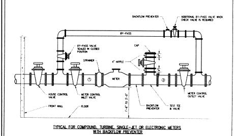
TYPICAL METER SETTING WITH BY-PASS
