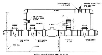
TYPICAL METER SETTING WITH BY-PASS TYPICAL FOR COMPOUND, TURBINE SINGLE-JET OR ELECTRONIC METERS WITHOUT BACKFLOW PREVENTER
