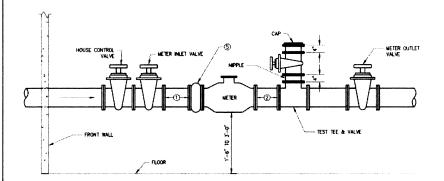
TYPICAL FOR COMPOUND, TURBINE SINGLE-JET, AND ELECTRONIC METERS WITHOUT BACKFLOW PREVENTER
