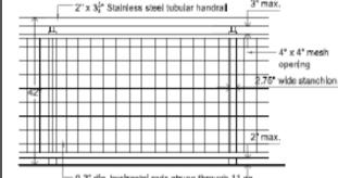
0.2" dla. horizontal rods strung through 11 ga vertical plates; bead-blasted stainless steel
