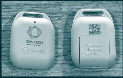
[FIGURE 12 ▲ ] Singapore's BLE-based exposure tracking "tokens." Photo: Roland Turner, CC BY-SA 3.0
