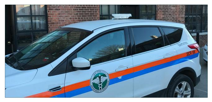
[FIGURE 15 A ] An MIT CityScanner sensor node on top of a New York City Department of Sanitation vehicle.
