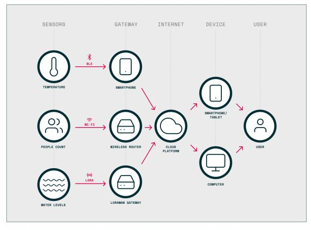
[FIGURE 04 **A** ] An example of basic IoT system architecture
