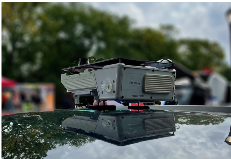
[FIGURE 04 ◀ ] CityScanner node on car mounted on NYC fleet vehicle. Photo: CityScanner
