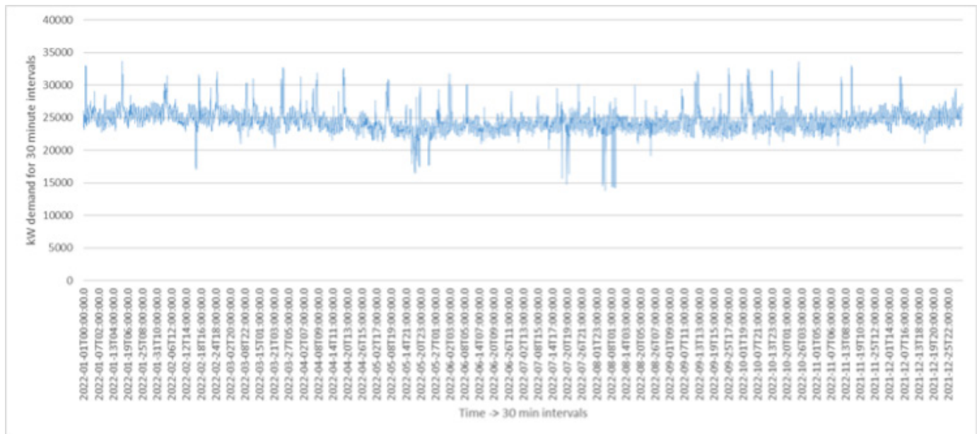
Figure 10. Aggregated load profile of the four above WRRFs, to approximate new WRRF's load.
