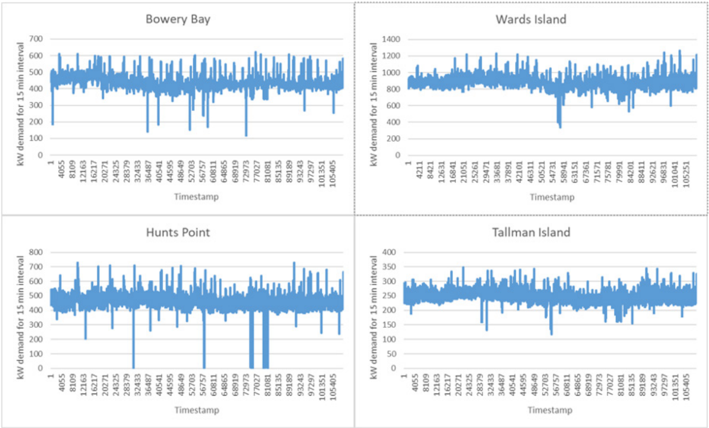
Figure 9. Load profiles of four existing New York City WRRFs to be consolidated by a Rikers Island WRRF.
