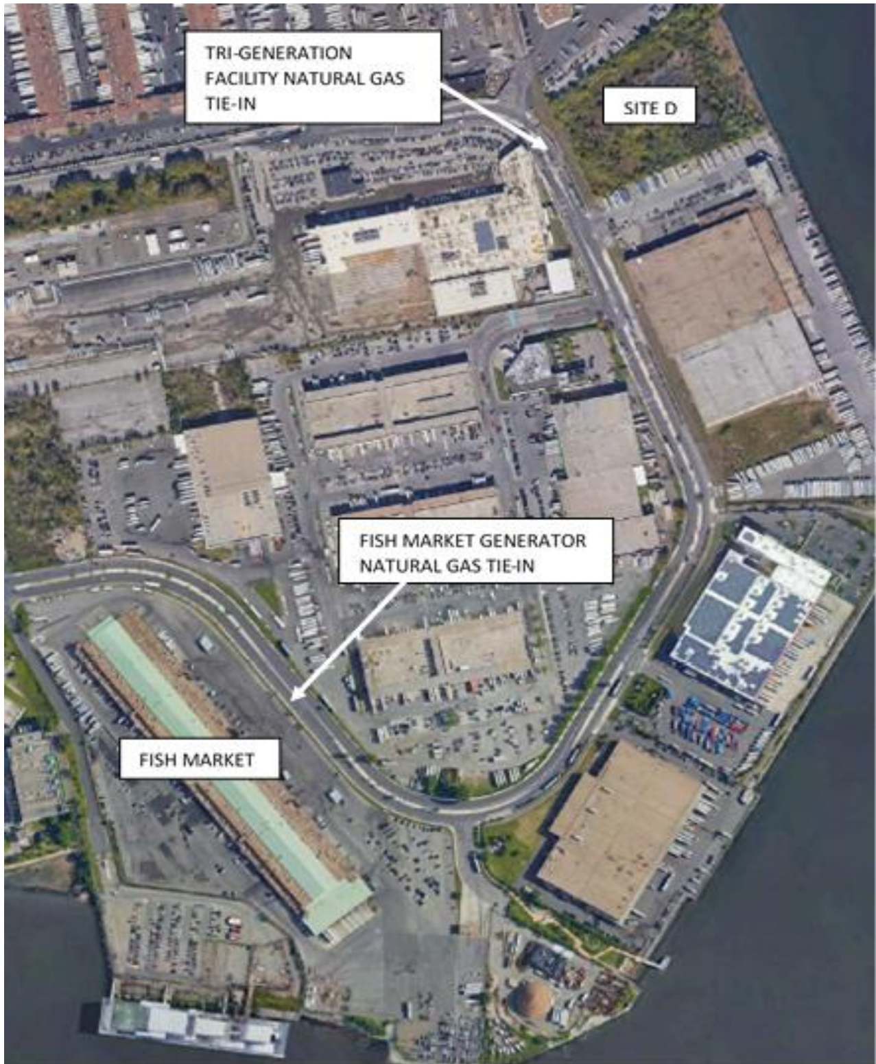
Figure 1-4. Natural Gas Tie-In Locations
