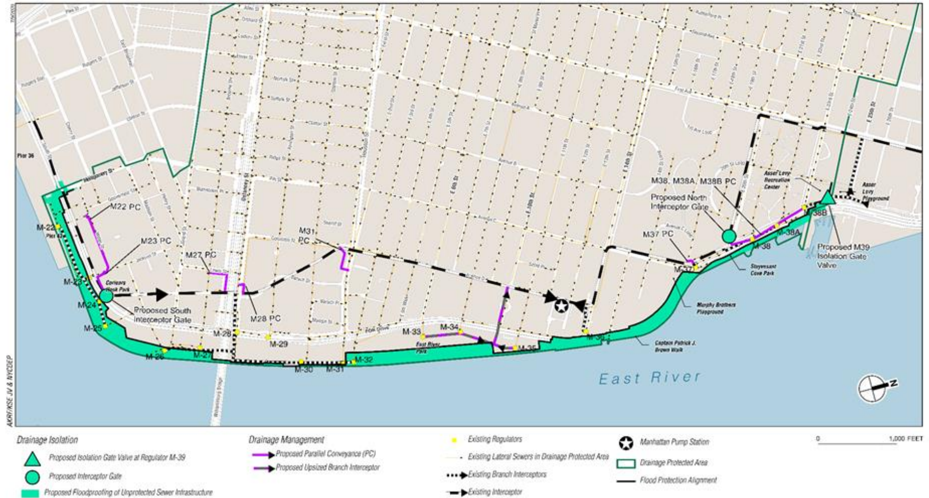
Figure 6—Drainage Isolation and Management Components
