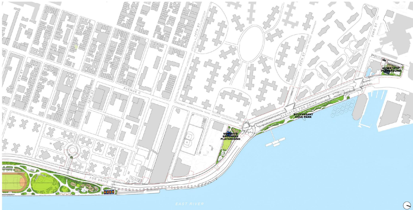
Figure 7b —Schematic of Preferred Alternative: Flood Protection System with a Raised East River Park
