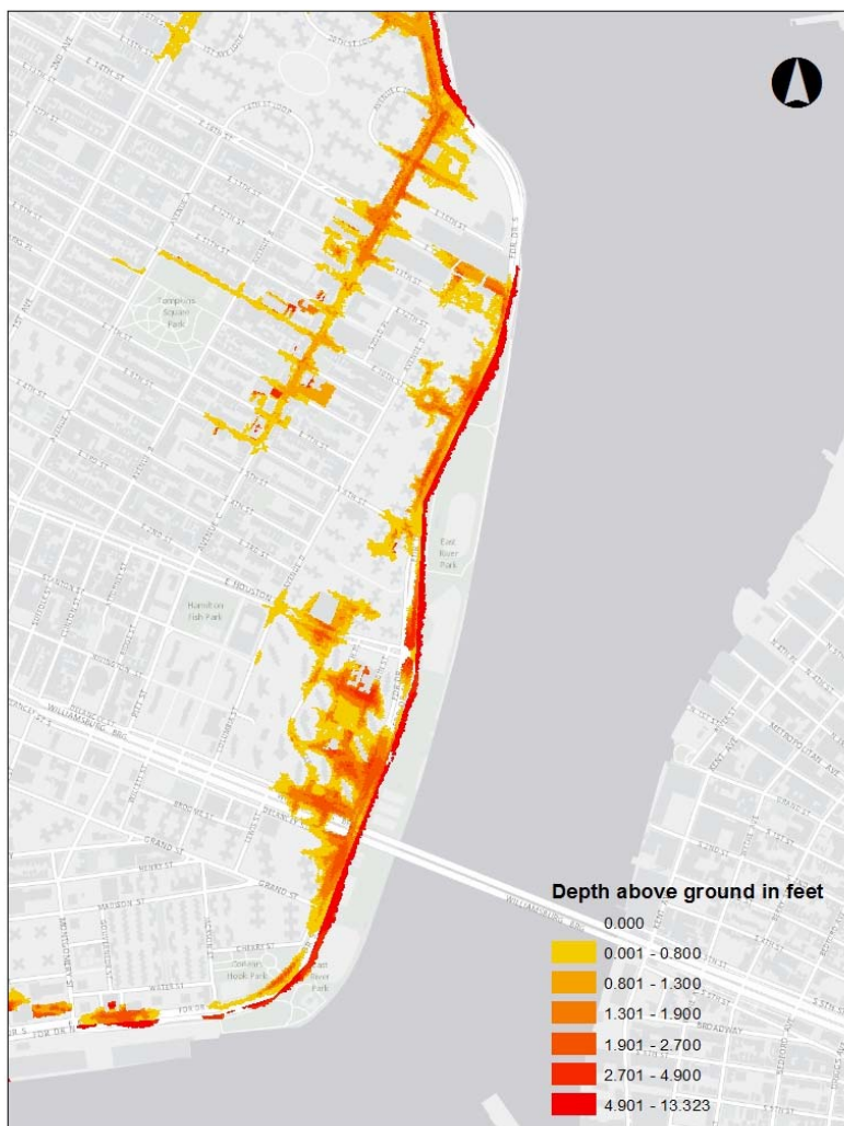
Figure 7. Possible Surface Flooding for the 20 Percent Annual Chance, 24 Hour Rain Event, Plus 1 Percent Annual Chance Storm Surge, Including SLR, Flood Protection System in Place and Without Drainage Management Elements
