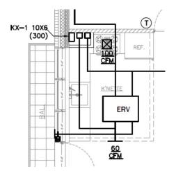
All drawings should clearly indicate unit type and location with duct type and location. Each plan must show area served with CFM indicated.
