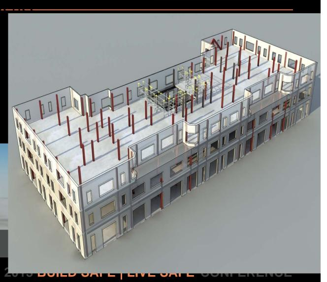
Provide shoring at all interior columns from above splice to underside of 2<sup>nd</sup> floor. **Shoring not shown in illustration (3d)**
