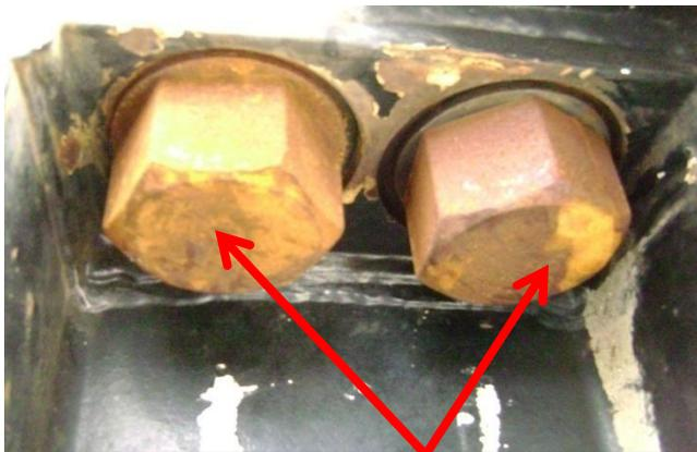
Markings hard to read due to corrosion
