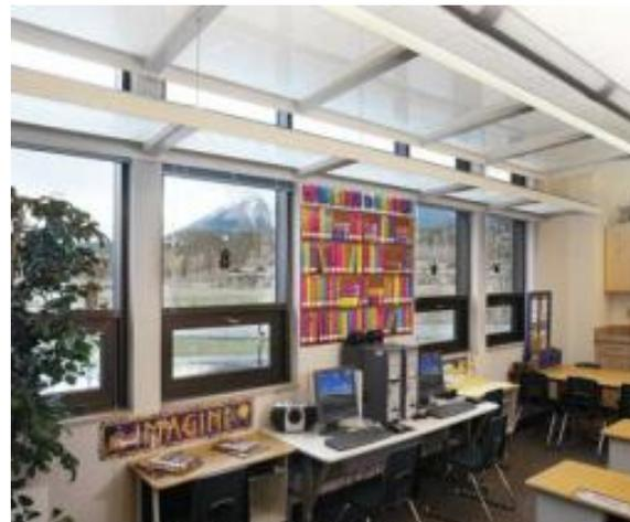
Figure LE-5.b. Daylight zone with automatic controls Exempt from Light-Reduction Controls
