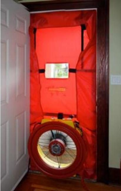
Figure BE-5. **Blower door installed for air leakage testing at a construction site**
