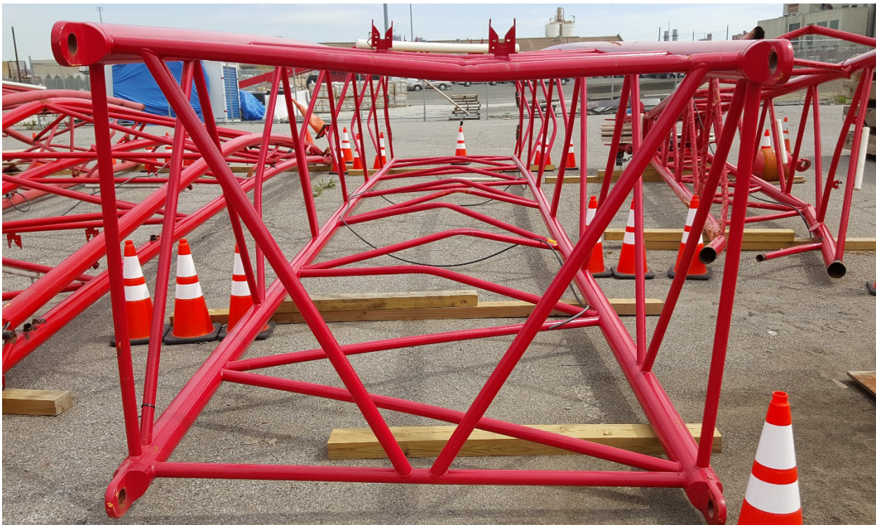
Photo 5 – Typical jib section J6
