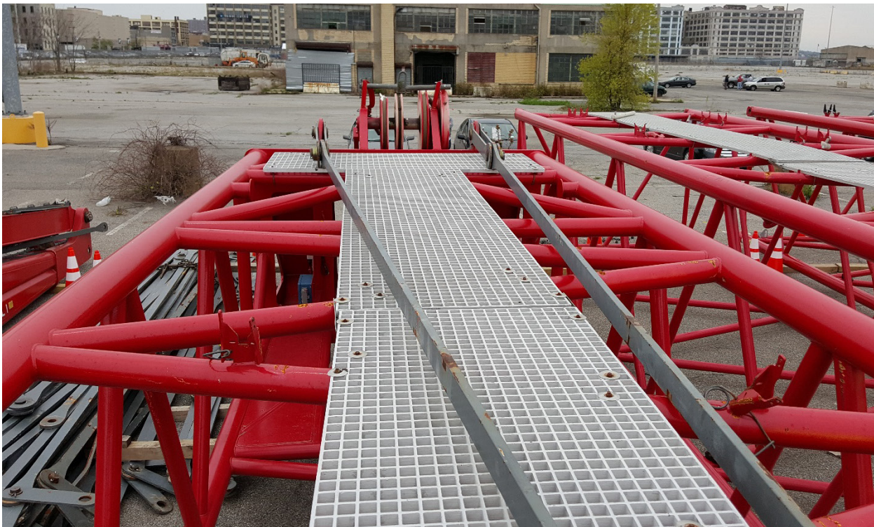
Photo 2 – FRP grating panel fastened to boom head
