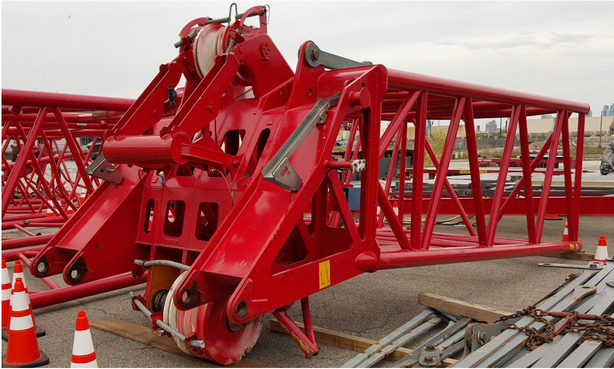
Photo 6 –Boom head (boom section B6)
