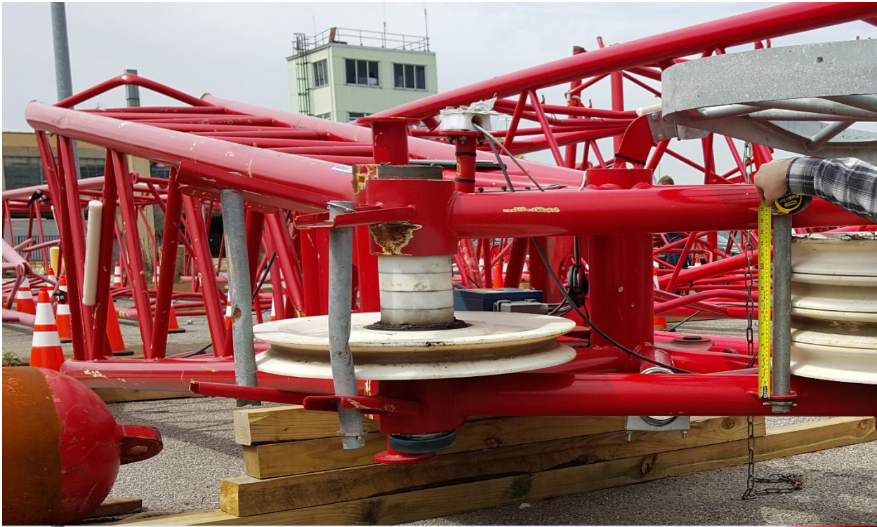
Photo 8 –Jib head (jib section J11) viewed from beyond tip
