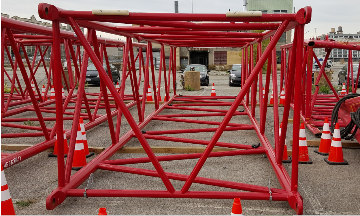
Photo 4 – Typical boom section B3
